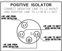
THE EARTH TERMINAL PROVIDED IS FOR CONTINUITY OF EARTH WIRING OR SCREEN, CONNECTION TO THIS TERMINAL IS NOT REQUIRED FOR OPERATION OF THE BASE OR ISOLATOR CONNECTED TO IT. CONNECTION TO THIS TERMINAL DOES NOT INFER EARTHING OF ANY PART OF THE BASE OR ISOLATOR CONNECTED TO IT.
